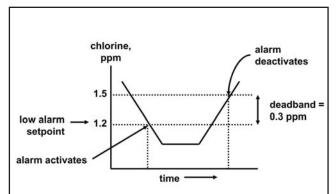
**FIGURE 5-2.** Low alarm logic. The alarm activates when the chlorine concentration drops below the low setpoint. The alarm remains activated until the reading increases above the value determined by the dead-band.
